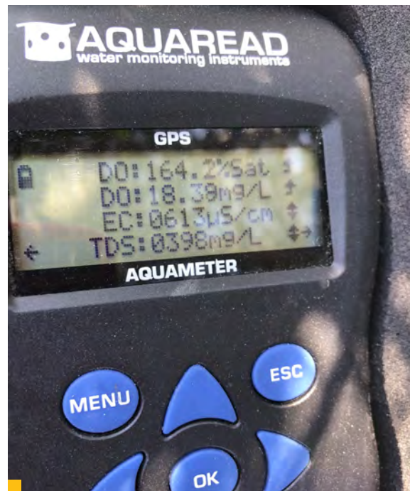
9 Aquaread – meranie in situ parametrov
