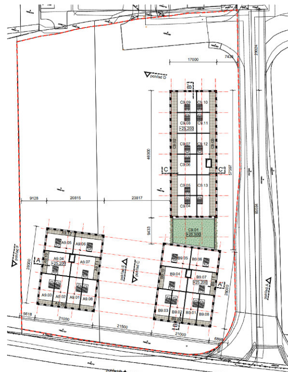
The architectural floor plan shows a building complex with three main sections labeled A, B, and C. Section A is a small rectangular building with rooms A8.01 to A8.07. Section B is a larger rectangular building with rooms B8.01 to B8.09. Section C is a long, narrow rectangular building with rooms C8.01 to C8.15. The plan includes dimensions, a north arrow, and a scale bar. A red dashed line outlines the perimeter of the building complex.
