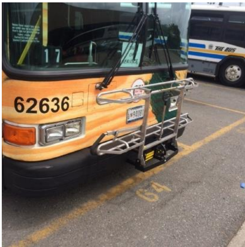
A picture 15-18 Folded bicycle carrier on the front bumper of the bus (Source: http://www.ridesmartsolutions.com )
