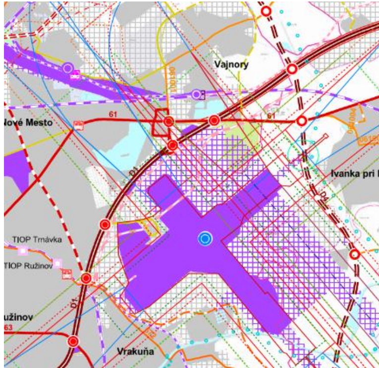
A picture 4-2 Connection of MR Štefánik Airport to railway lines (Source UPN R BSK as amended)
