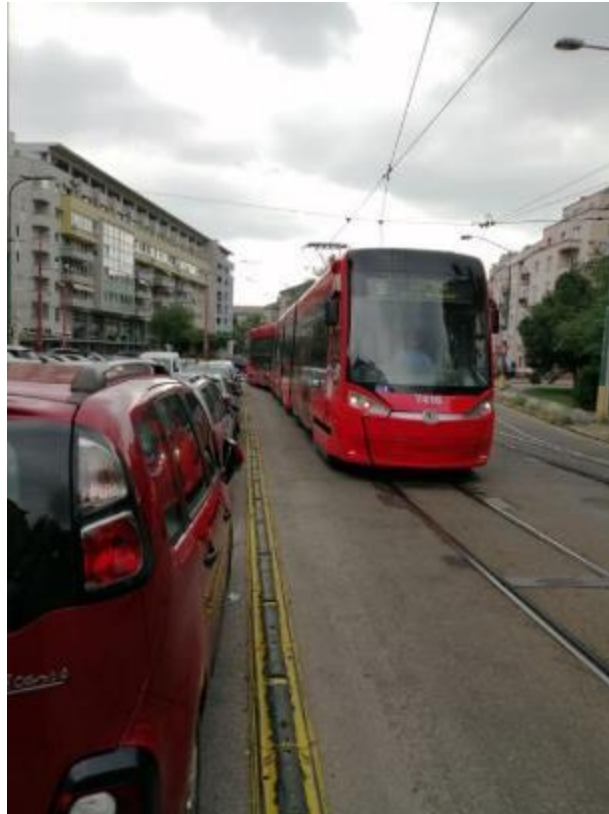
A picture 5-1 Tram body protection by guiding threshold (Source: Processor)
