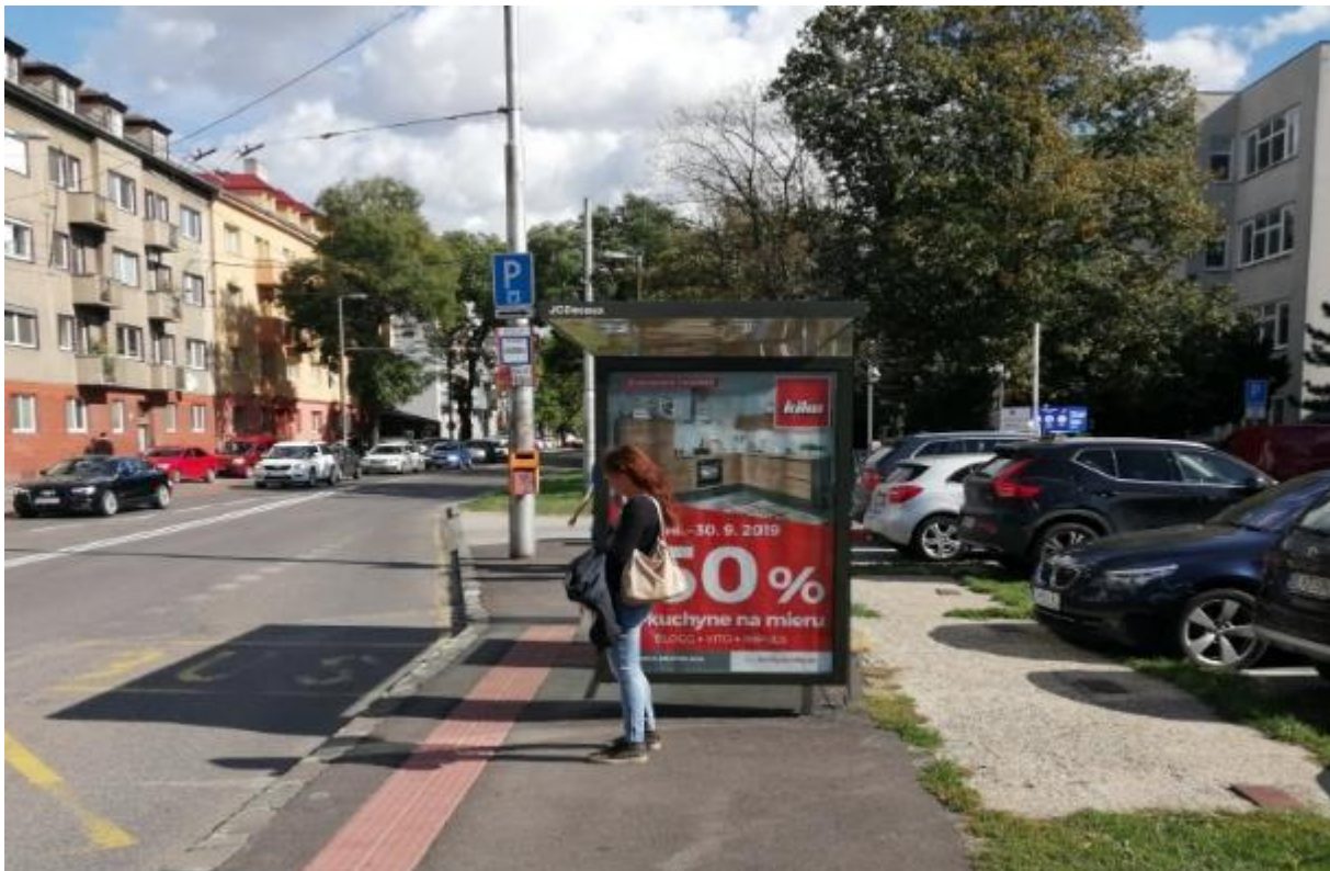
A picture 12-3 Improperly located shelter at a public transport stop. There is space to place it behind the edge of the sidewalk. At the same time, the design of the shelter with an opaque side wall filled with advertising on the side of the arrival of the public transport vehicle is also inappropriate (Source: Processor)
