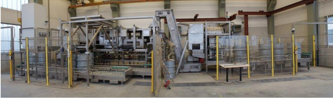
*Figure 7: Soil measuring system (right material application, left measurement and separation)*
